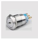
Diameter: Ø 19mm Color: R, G, Y, O, B, W Switch Rating: 5A/250VAC Contact Configuration: 1NO 1NC/
